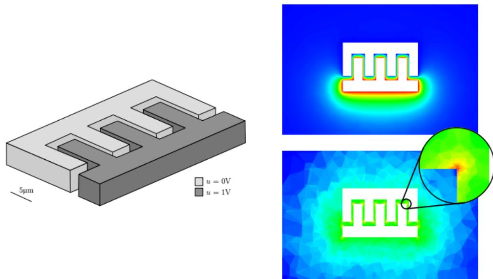
**Figure:** Geometry (left), numerical solution (right, top) and final adaptive mesh (right, bottom) for the comb-drive actuator test case [Di Pietro and Specogna, 2016]
