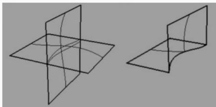
represented by b-spline curves in the parameter domains of the two surfaces and/or by their image on the two surfaces.
