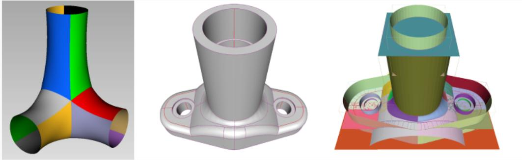
Geometric model made of patches, glued together along intersection curves.
